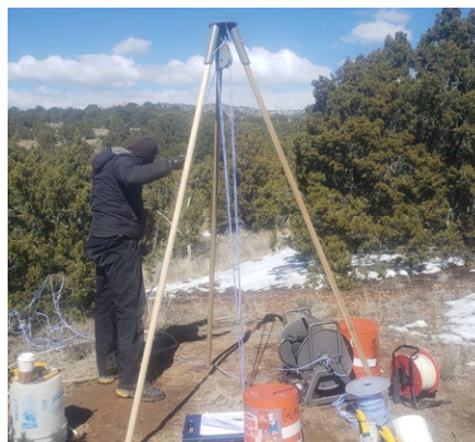
DBS&A staff conducted aquifer pumping tests to assess reasonable flow rates for groundwater extraction.
