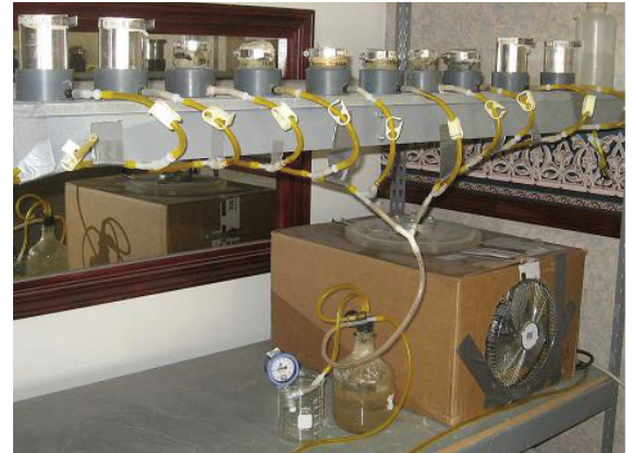
A vacuum is applied to the group of saturated samples in a parallel configuration
