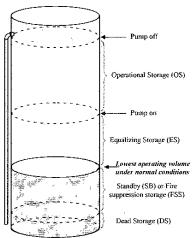
When calculating **Contact Time**, use the <u>lowest volume of water</u> in the tank under peak flow conditions: DS + (SB or FSS)
