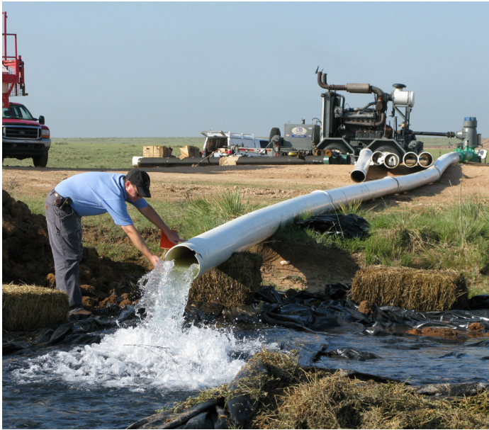
Prototype supply wells demonstrated production capacities ranging from 850 to 1,140 gallons per minute.
