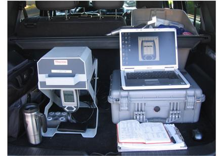
On-site analysis of metals with XRF
